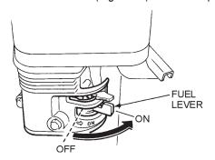
Figure 11. Fuel Valve Lever
